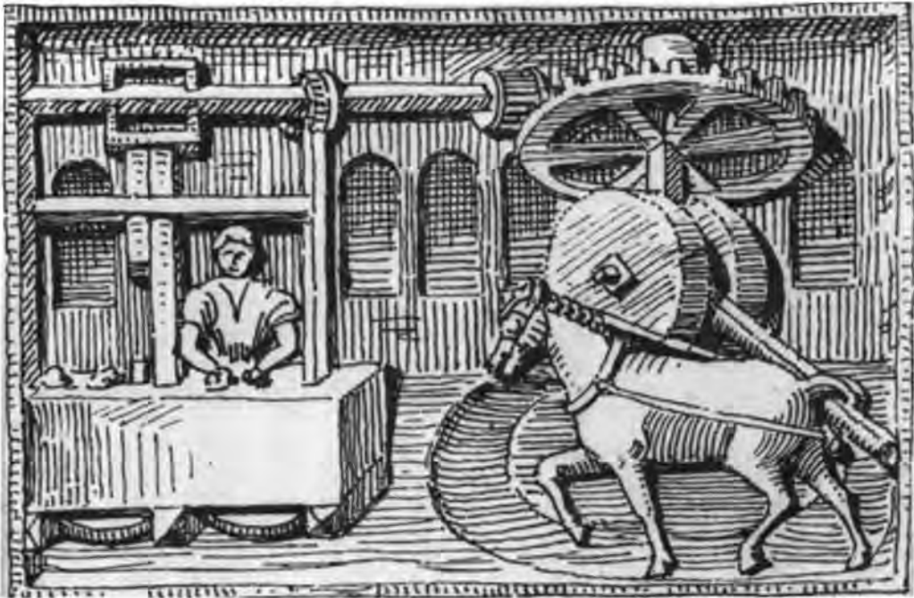
33. Horse-drawn oil-press with upright mill-stones, façade stone (p. 181 n. 182)
