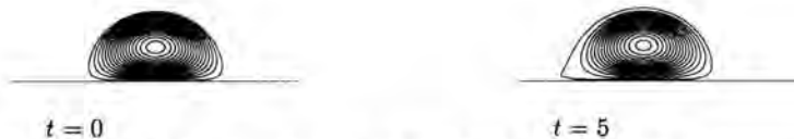
Fig. 2. The evolution of the unperturbed Lamb dipole for Re = 1000 from t = 0 to t = 5 (in non-dimensional time units) shown by vorticity contours \Delta\omega = 0.5 ; only the upper half-plane is shown.
