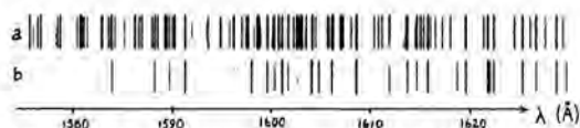
Fig.1. Hollow cathode spectra of Y run with a) Ar and b) Ne as a carrier gas.
