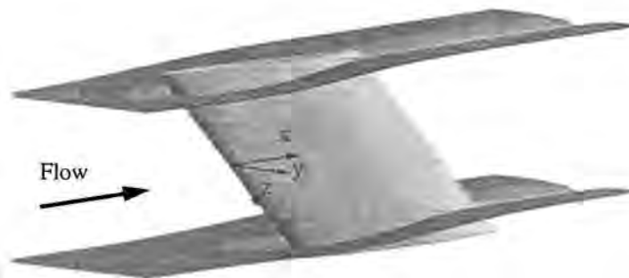
Figure 1: 45° swept wing with wall liners at the Arizona State University Unsteady Wind Tunnel.
