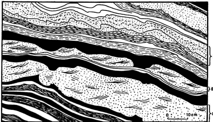
Fig. 15. Irregular bedding due to pull-apart (bed B, with current bedding) and slump structure (bed C with current bedding, etc.), convolute bedding (bed A), in alternating shales, siltstones and fine grits (from photograph). Upper Llandoveryan south of Aberystwyth.
