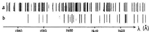
Fig.1. Hollow cathode spectra of Y run with a) Ar and b) Ne as a carrier gas.
