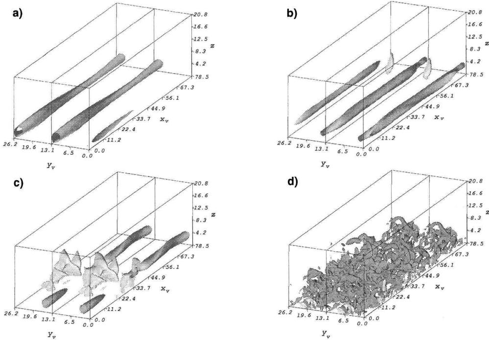
Figure 3: Visualization of vortical structures by isosurfaces of low static pressure. For visualization twice the computational domain in the spanwise direction  $y$  is shown. a):  $t = 800$ ,  $p_{iso} = -0.0022$ ; b):  $t = 920$ ,  $p_{iso} = -0.0031$ ; c):  $t = 970$ ,  $p_{iso} = -0.004$ ; d):  $t = 1300$ ,  $p_{iso} = -0.005$ .
