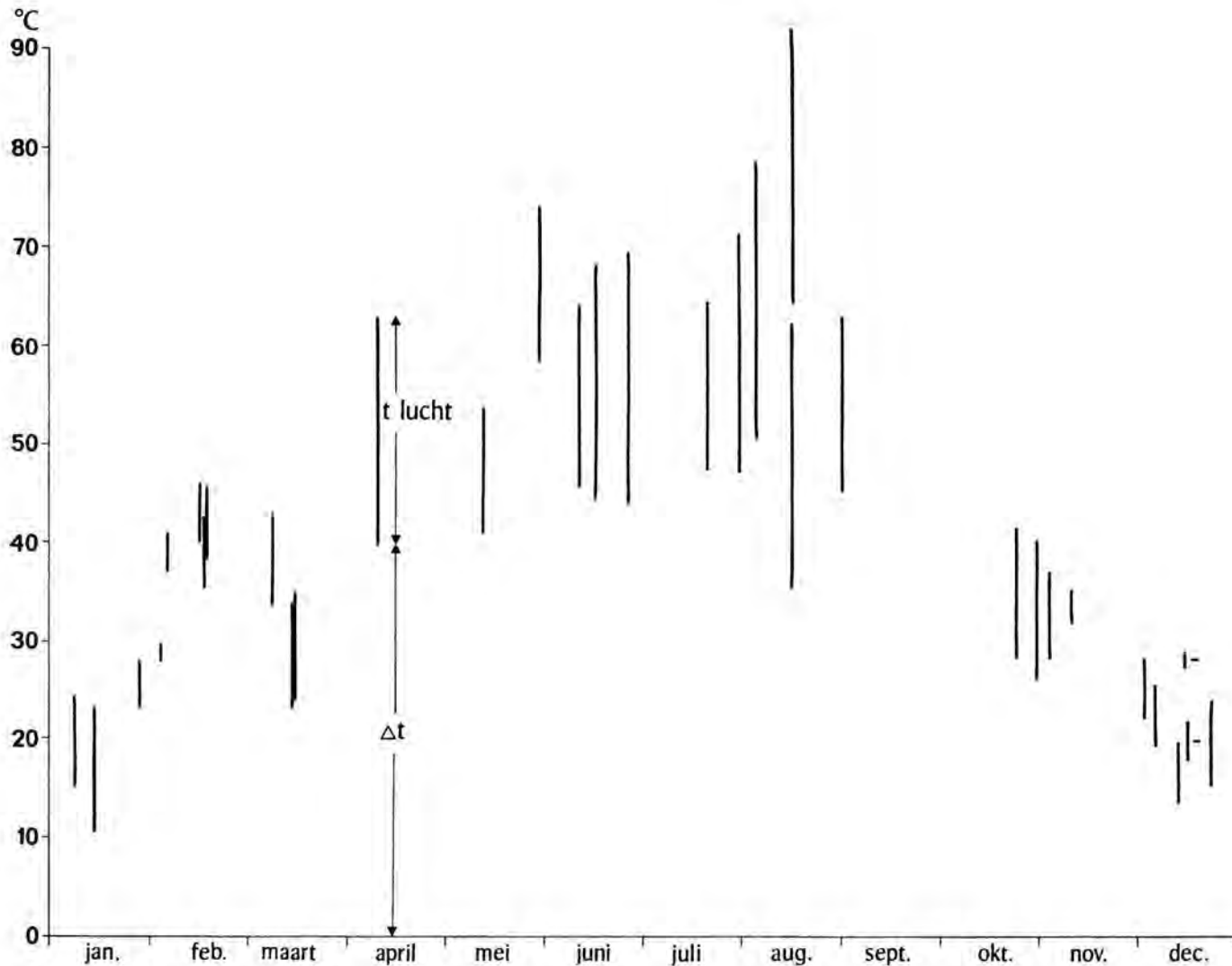
Fig. 6. High surface temperatures over the year. The top of the bar indicates the observed temperature, the length, the air temperature and the lower end the difference between surface and air temperature ( \Delta t ). When air temperatures are negative (indicated by a minus sign) \Delta t is indicated by the top and the surface temperature by the bottom of the bar.
