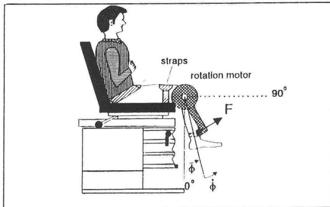
**Figure 1.** Schematic of experimental set-up. The angular position and velocity, measured at the motor axis, are defined positive in extension motion with zero as indicated. The patient is strapped at the hip and above the knee to measure knee torque (at the tibia) only and to ensure static position of the body.
