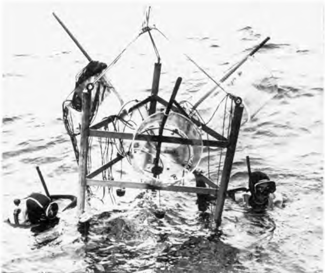
Plate I. Lowering of the scuba operated beljars for the determination of the community metabolism. This metabolism is measured by recording the oxygen production and consumption rates of sediment and phyto and zoobenthos over a 30 hours period.
