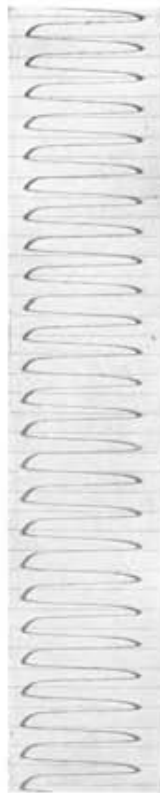
Fig. 3. Electrode 1.4 cm. long, of a diameter of 3 mm., not sealed in, solution as in the experiment in fig. 1. Potential measured at the bottom of the electrode. Current density 32—36 milli-ampère/cm 2 . 1 period 5.25 sec.
