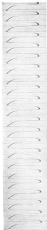
Fig. 1. Sealed-in iron electrode 1.5 cm. long, of a diameter of 3 mm. Solution contains per Liter 0.72 gr. mol. \text{FeSO}_4 \pm 0.014 gr. mol. \text{FeCl}_2 . Potential measured halfway the height. Current density 28—33 milli-ampère/cm 2 . 1 period 6.15 seconds. Difference of the extreme values \pm 1.7 Volt.
