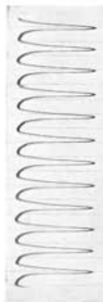
Fig. 3. Electrode 1.4 cm. long, of a diameter of 3 mm., not sealed in, solution as in the experiment in fig. 1. Potential measured at the bottom of the electrode. Current density 32—36 milli-ampère/cm 2 . 1 period 5.25 sec.
