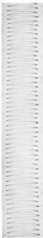
Fig. 4a. Iron electrode 5.3 cm. long of a diameter of 3 mm. not sealed in. Solution as in the experiment in fig. 1. Potential measured 1.5 cm. from the bottom. Current density 38—43 milli-ampère/cm 2 . 1 period 2.7 seconds.
