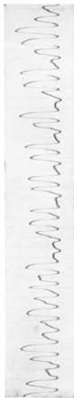
Fig. 6. Electrode and solution as in fig. 5. Potential measured 1 mm. under the liquid level. Current density 47—53.5 milli-ampère/cm 2 . 1 period 3.65 seconds.
