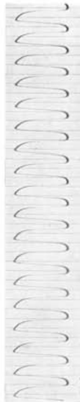
Fig. 1. Sealed-in iron electrode 1.5 cm. long, of a diameter of 3 mm. Solution contains per Liter 0.72 gr. mol. \text{FeSO}_4 \pm 0.014 gr. mol. \text{FeCl}_2 . Potential measured halfway the height. Current density 28—33 milli-ampère/cm 2 . 1 period 6.15 seconds. Difference of the extreme values \pm 1.7 Volt.
