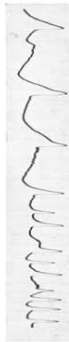
Fig. 7. Electrode \pm 60 cm. long of a diameter of 3 mm. electrode spirally wound in 5 windings. Potential measured at the second winding from the top. Strength of the current regularly periodical at \pm 0.5 ampère.
