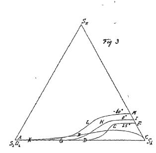
This line is ABC in figure 3, the part BC is extrapolated, except the point C. From this line we find for the solubility curves at 25° DFF, at 0° GHI, at -60° KLM.
