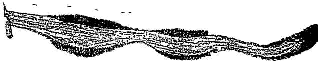
Fig. 5. Longitudinal section of a fibre as mentioned in fig. 3. One sees that the circular fibrils only appear in some places of the fibre. (enlargement 60).
