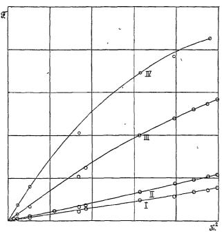
Curve I refers to 20.'3 K. curve II to 14,°7 K, III to 4.°25 K. and IV to 1.°9 K. Each division along the horizontal axis corresponds to about 90 kilogauss, along the vertical axis to 25 grammes. The ratio of the force to the square of the field on the axis of the poles per unit of susceptibility was about ½, neglecting small changes in the topography of the field.
