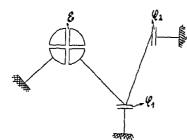
They were 7—8 cm. long, 2 cm. broad and 0.06 cm. thick. The two broad, sides were coated with tin <sup>1</sup>). One of the tin coatings of each plate was earthed, the two others were metallically connected with one another and with one pair of quadrants of the electrometer, as is shown in the figure.
