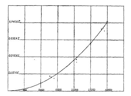
Inspection of the figure or a simple calculation easily shows that the quadratic law is obeyed within the limits of the errors of observation of the measured displacements. The magnitude of the displacement has been measured in the average in each of the ten points to within 0.002 or 0.003 Å.U.
