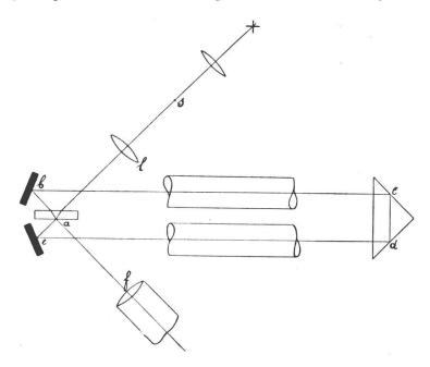
The above figure is reproduced from an earlier paper<sup>1</sup>) on FRESNEL'S convection coefficient for light of different colours in water, in which use is made of MICHELSON and MORLEY'S interferometer. In a the ray meets MICHELSON'S slightly silvered mirror. There the
